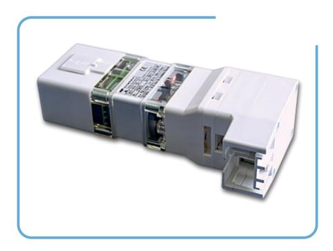
The EasyTrack Plus motors are an easy and affordable way to motorize smaller and lighter curtain tracks. The curtain is being transported by a textile transport or toothed drive belt. In case of emergency it can also be moved by hand – without any damage to the system or recalibration.
